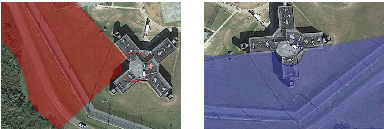
Figure 2 - Rendering of the Spynel-M's capabilities and customizable options: sector scan rates at both 90° 2.5 Hz for 2.5 scan/second (left) and 180° 1.5 Hz for 1.5 scan/second (right) and the potential ranges over a prison site.
